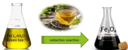
Figure 1. Synthesis of \text{Fe}_3\text{O}_4 -GTE NPs.
