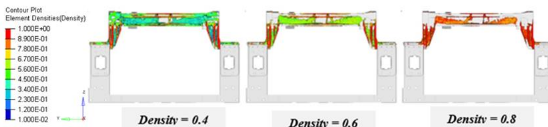
Figure 4: Optimization results of first design volume under various iso-contour
