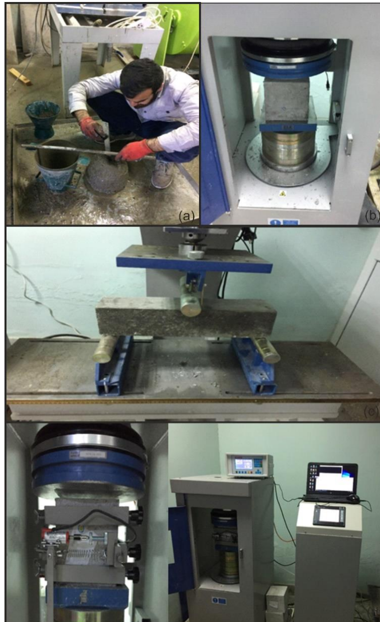
Figure 2. Tests conducted in this study (a) slump, (b) compressive strength, (c) flexural strength and (d) static modulus of elasticity
