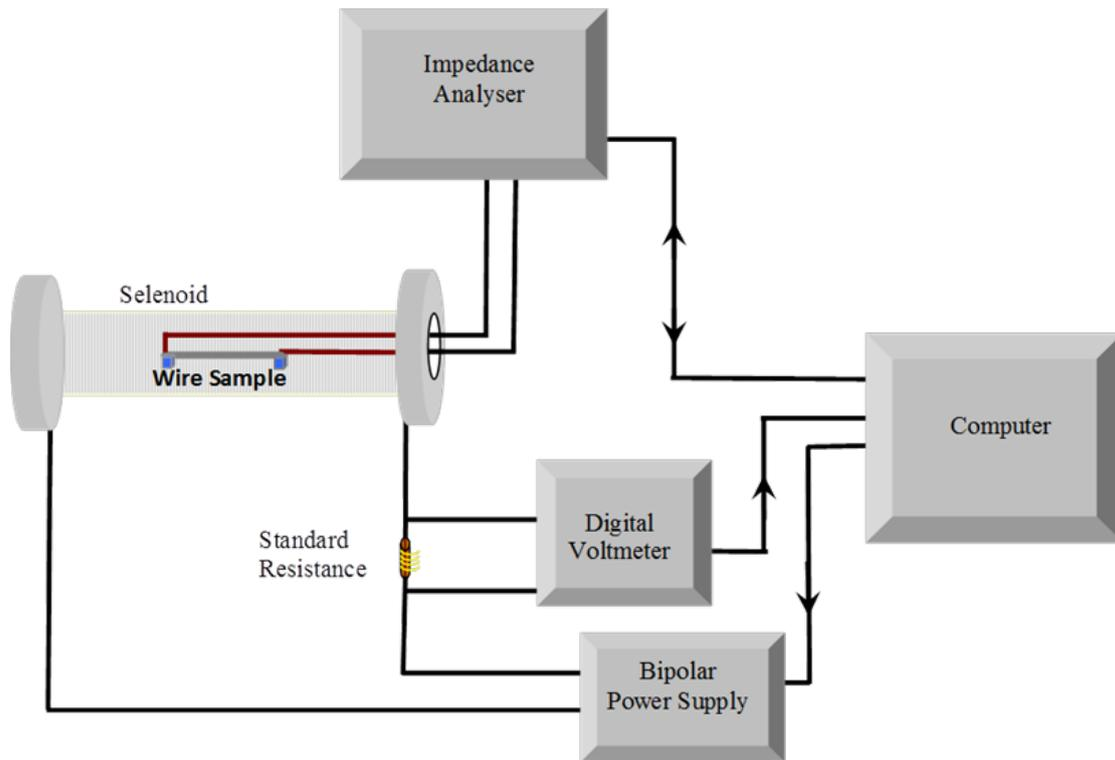
**Figure 1:** MI measurement system
