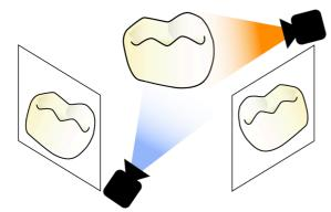
**Fig. 5.** Stereophotogrammetry is a technology that generates files by algorithm analyzing numerous pictures
