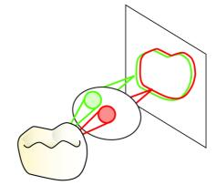
Fig. 4. AWS requires a circular path around the optical axis and produces a rotation of interest points
