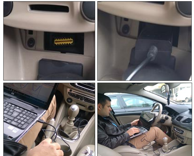
Figure 10. Data acquisition via OBDII
