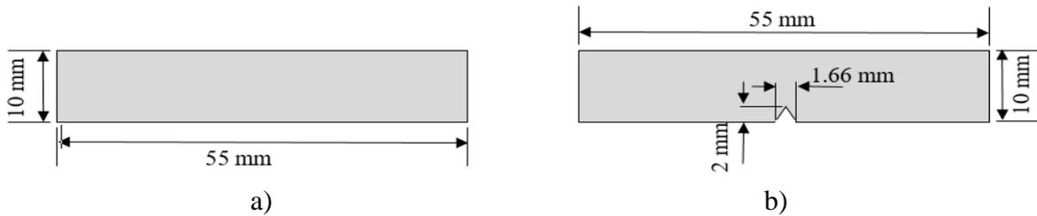
**Figure 5.** The dimensions of Charpy samples; a) unnotched for flatwise loading, b) notched for edgewise loading
