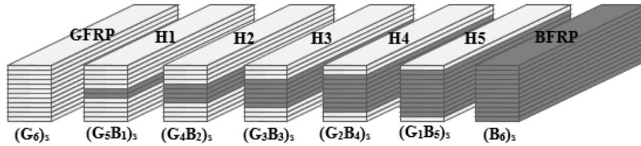
**Figure 1.** Stacking sequences of glass and basalt fabric layers.
