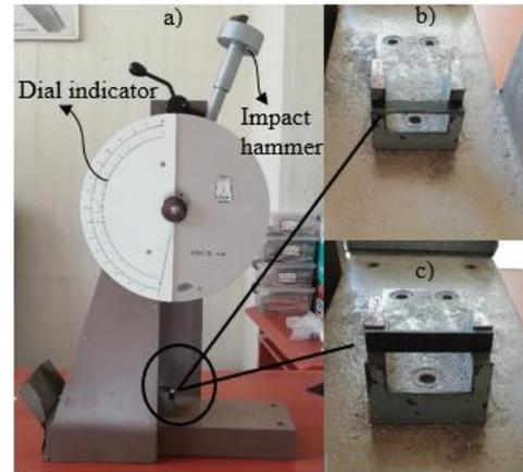
**Figure 3.** a) Köger 3/70 Charpy impact tester, b) edgewise placement, c) flatwise placement
