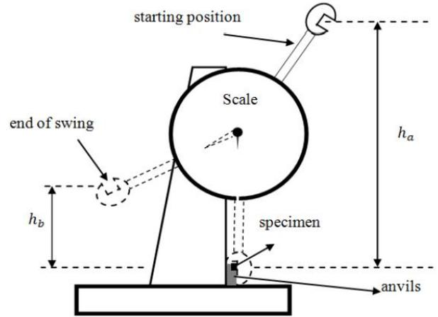
**Figure 4.** Schematic illustration of Charpy impact test
