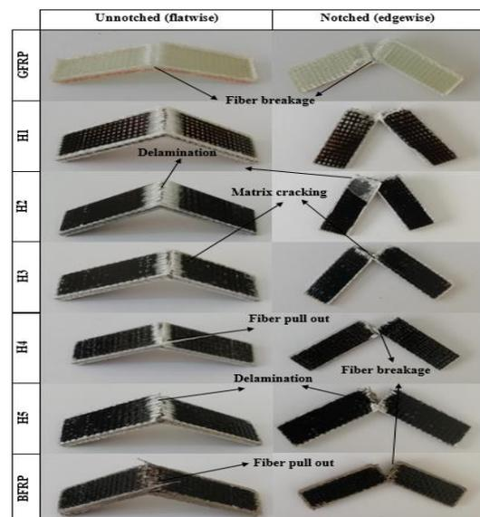
**Figure 8.** Damage shapes and failure modes of impacted samples
