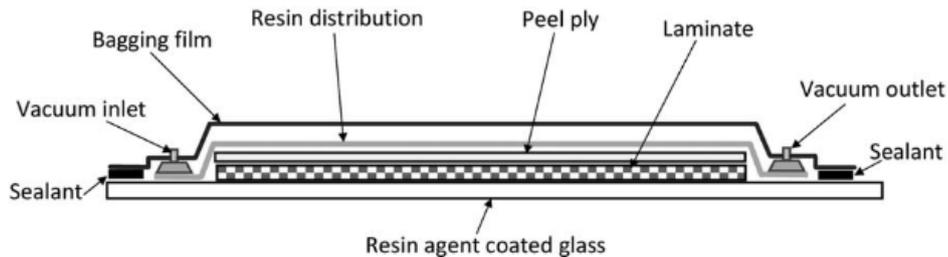
**Figure 2.** Schematic illustration of vacuum assisted resin transfer molding [11]
