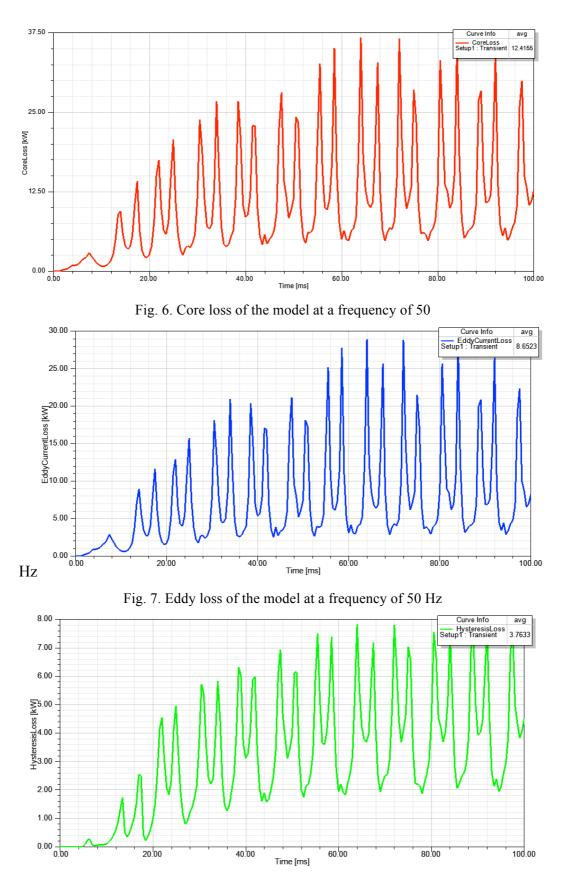
Fig. 8. Hysteresis loss of the model at 50 Hz frequency
