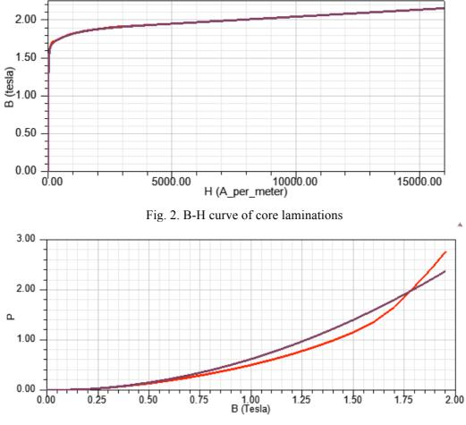
Fig. 3. P-B curve of core losses
