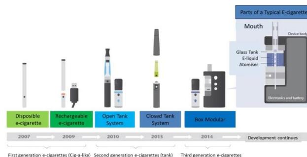
**Figure 1.** Change of e-cigarette design over time; each e-cigarette on the figure shows that e-cigarettes change over time from single-use to reusable cigarette-like e-cigarettes, from second generation electronic cigarettes to open and closed tank/cartridge systems, and finally to third generation modular e-cigarette devices (1).
