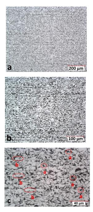
**Figure 1.** Microstructure of non-microalloyed steel (EN 10025-2:2004 S275JRC (RSt37-2)) ( in figure c a : acicular ferrite b : pearite)
