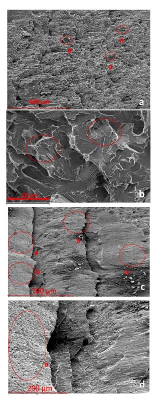
Figure 4. Fracture surfaces of samples (a, b Nb-added steel, c and d Nb-Ti added steel) ( in figure c and d, a : dimple ductile fracture )
