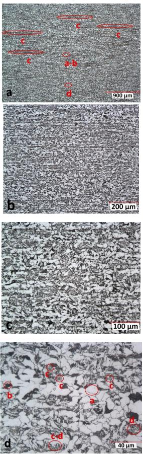
Figure 3. Microstructure of Nb-Ti added microallyed steel (EN 10028-3 - P355NH (WStE 355)) ( in figure a,d a : ferrite b : pearite c : Ti[C,N] d : NbC )
