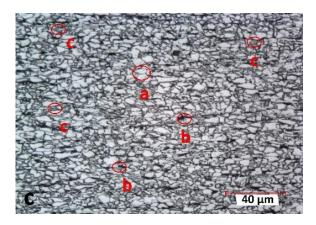
Figure 2. Microstructure of Nb-added microallyed steel (EN 10149-2:2013 S355MC (QStE 380TM)) ( in figure c a : ferrite b : pearite c : NbC )
