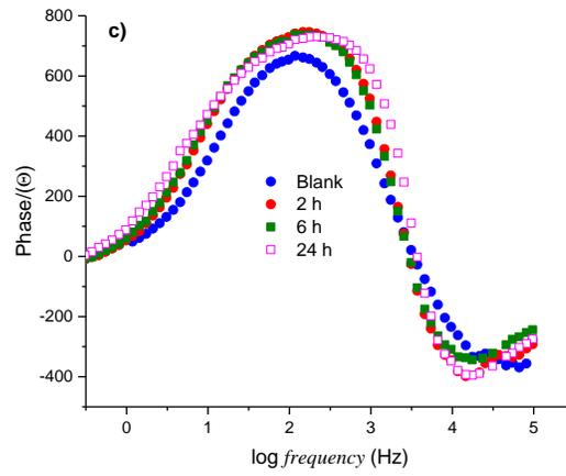
FIGURE 1. Electrochemical impedance curves of aluminum **a)** Nyquist **b)** Bode- $|Z|$  **c)** Bode-phase plots in the presence of *Cannabis sativa* L. extract in 0.5 M H<sub>2</sub>SO<sub>4</sub> with during 2 h, 6 h and 24 h.
