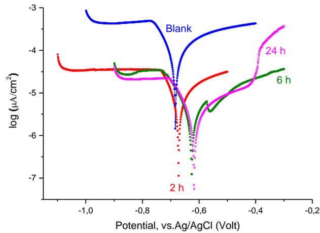
FIGURE 2. Potentiodynamic current potential curves of aluminum in 0.5 M H<sub>2</sub>SO<sub>4</sub> in the presence of *Cannabis sativa* L. extract with during 2 h, 6 h and 24 h.
