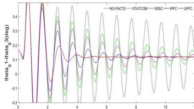
**Figure 13.** Difference of rotor angular positions of generator-1 and 3 for all cases.
