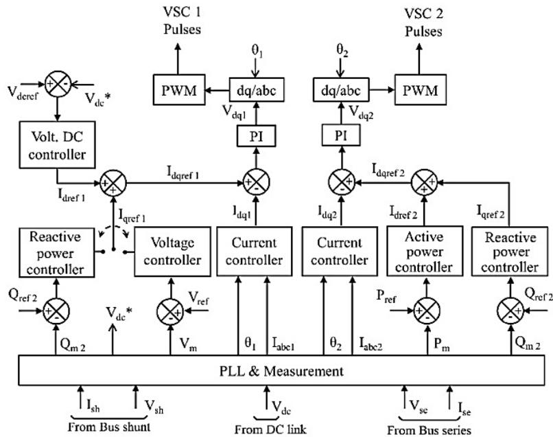
Figure 8. Basic control diagram of UPFC [6].
