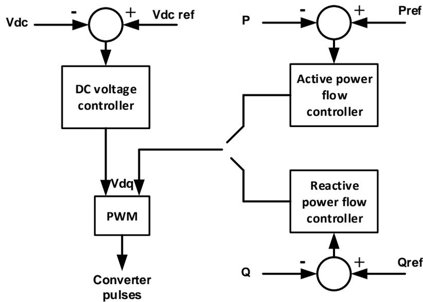
**Figure 4.** Basic control diagram of SSSC [6].
