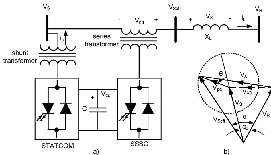
**Figure 7.** The simplified configuration of UPFC: (a) typical arrangement (b) voltage phasors [6].
