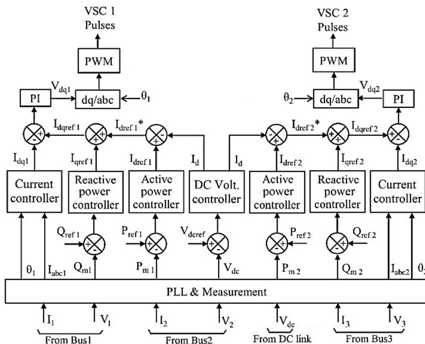
**Figure 6.** Basic control diagram of IPFC [6].
