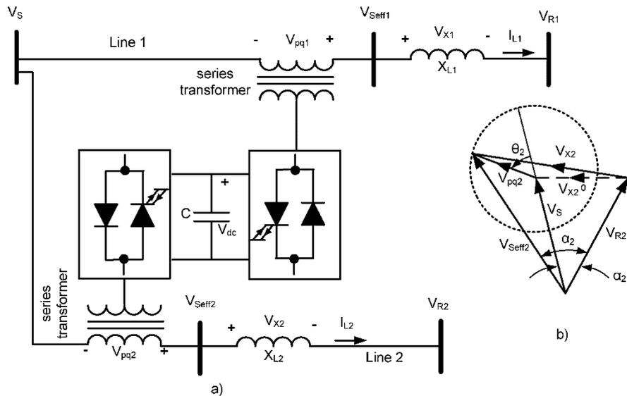
**Figure 5.** The simplified configuration of IPFC: (a) arrangement (b) voltage phasors [6].
