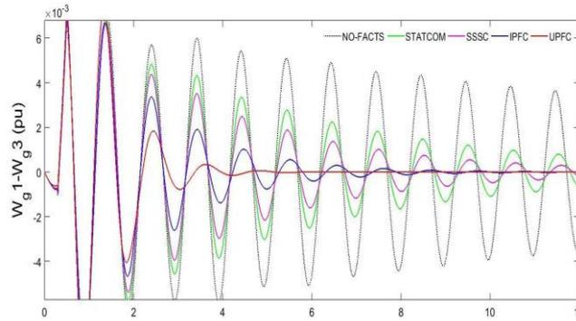
**Figure 12.** Difference of rotor angular speeds of generator-1 and 3 for all cases.
