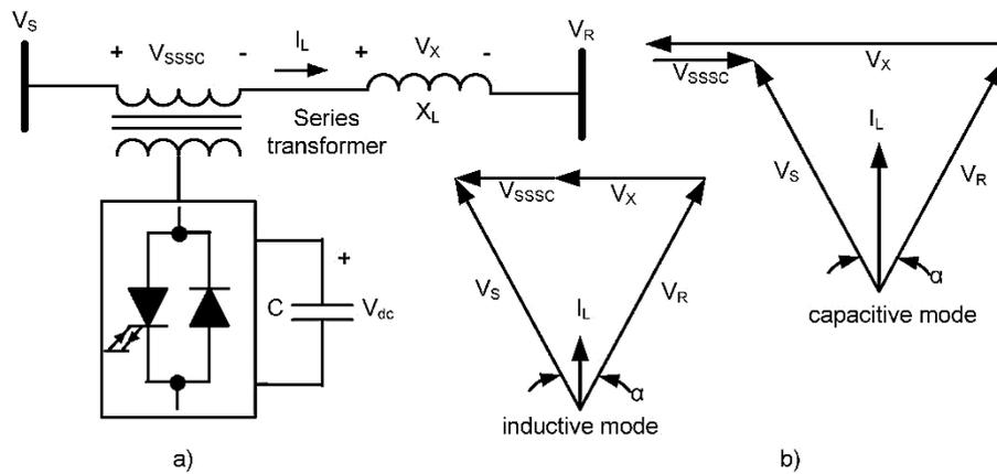
**Figure 3.** The simplified configuration of SSSC: (a) arrangement (b) operating modes [6].
