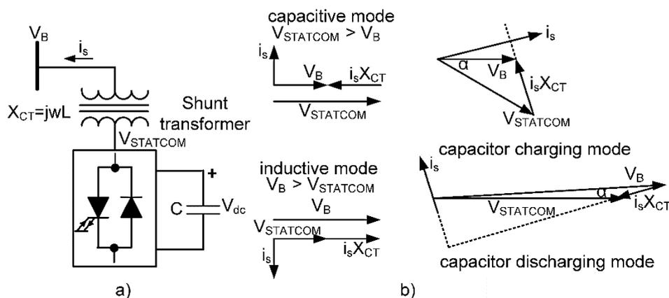
**Figure 1.** The simplified configuration of STATCOM: (a) arrangement (b) operating modes [6].
