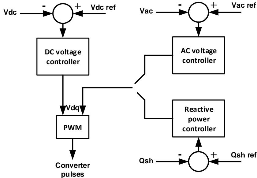
Figure 2. Basic control diagram of STATCOM [18].
