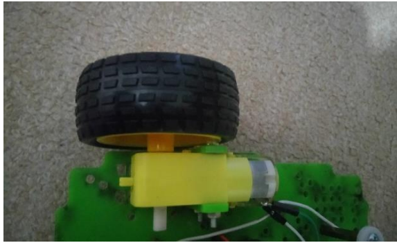
Figure 3. Image of the Left DC Motor and Wheel Integration to the Frame
