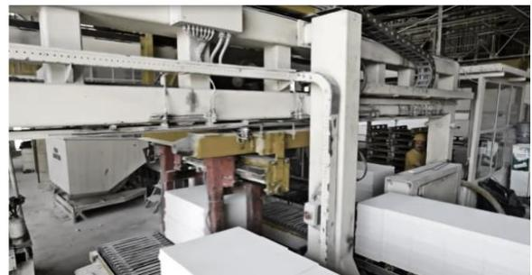
**Figure 4.** Extraction of AAC from autoclaves and separation from each other.
