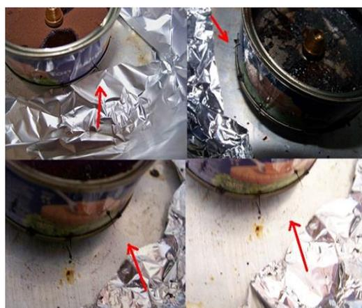
**Figure.8** The output of Lignin Fibers from the Perforated Chamber with Nozzle Function
