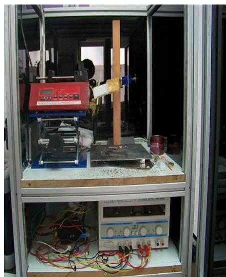
**Figure. 9** Electrospinning Fiber Production Device.
