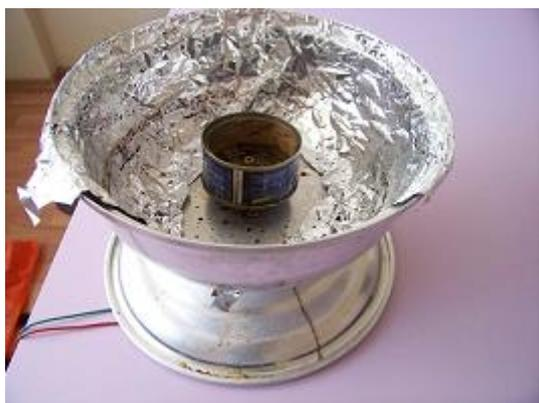
**Figure. 7** New Device Designed in the Scope of the Modification of Melt Fiber Extraction Method.
