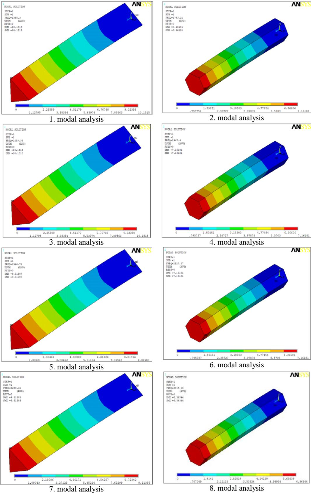
**Figure 3.** Fundamental frequency analysis for finite element approach.
