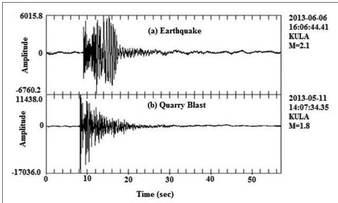
Figure 3- Vertical component velocity seismogram recorded at KULA station; (a) Earthquake, (b) Quarry Blast.
