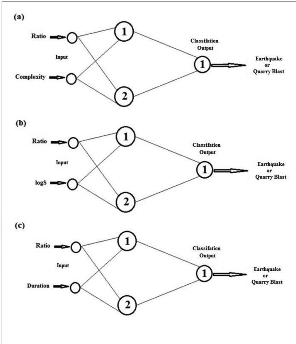
Figure 7- Artificial neural network structure for seismic events a) ratio versus C, b) ratio versus logS, c) ratio versus duration.
