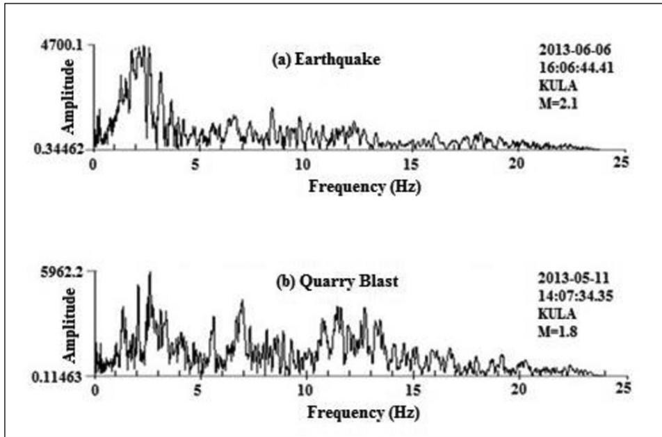
Figure 4- Normalized amplitude spectrum of the signal recorded at the KULA station; (a) Earthquake, (b) Quarry Blast.
