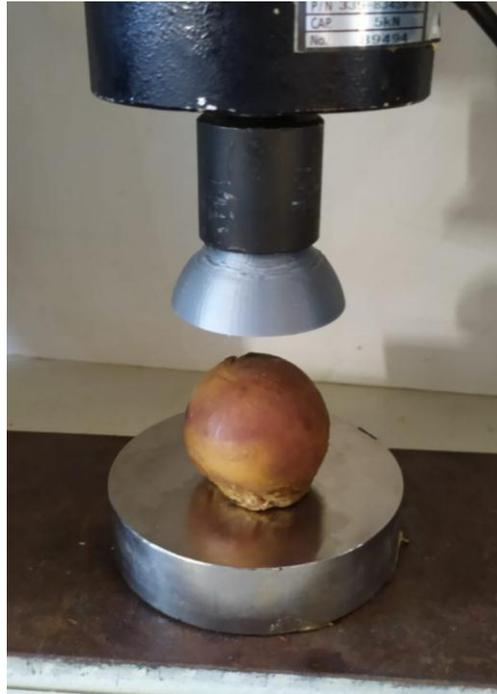
**Figure 1.** Compression testing set-up.
