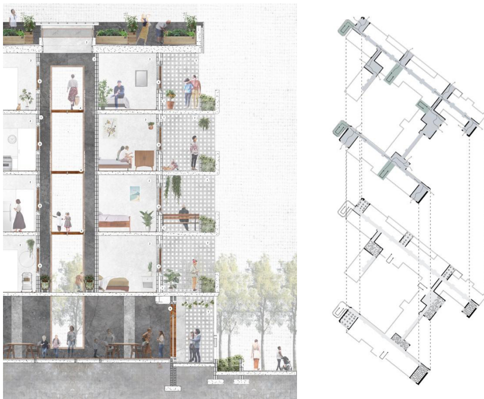
Figure 2. A section and a diagram of the adapted Helen Bowden Nurses Home showing the process of subtraction that allows for more social engagement on and across levels (Bezuidenhout 2017).
