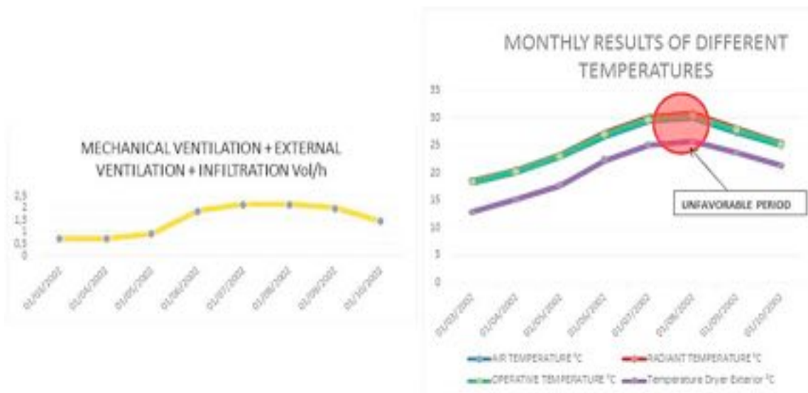
Graph 01 and 02. Ventilation and different temperatures for the old state during the summer period
