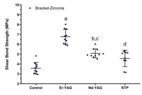
**Figure 1.** Values of shear bond strength between orthodontic brackets and zirconium oxide infrastructures treated with Er:YAG, Nd:YAG, and KTP lasers. Data were expressed as mean (midline) and SD (whiskers). <sup>a</sup>P<0.05, Er:YAG group vs. Nd:YAG, KTP, and control groups . <sup>b</sup>P>0.05, Nd:YAG group vs. KTP group. <sup>c</sup>P<0.05, Nd:YAG group vs. control group. <sup>d</sup>P<0.05, KTP group vs. control group.
