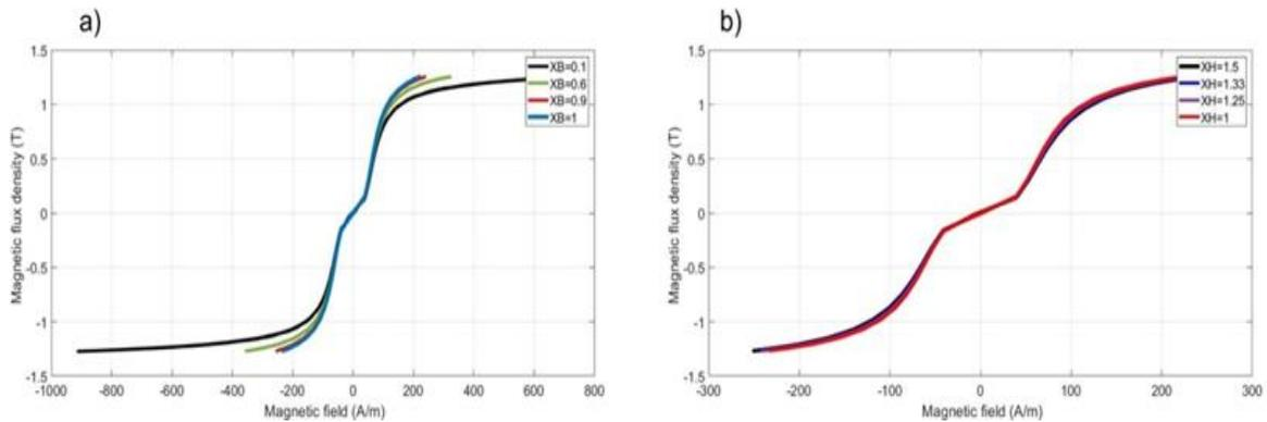
**Figure 10.** Overall B-H curve of the ring-core with different values of: **a)**  $X_B$  and **b)**  $X_H$ .
