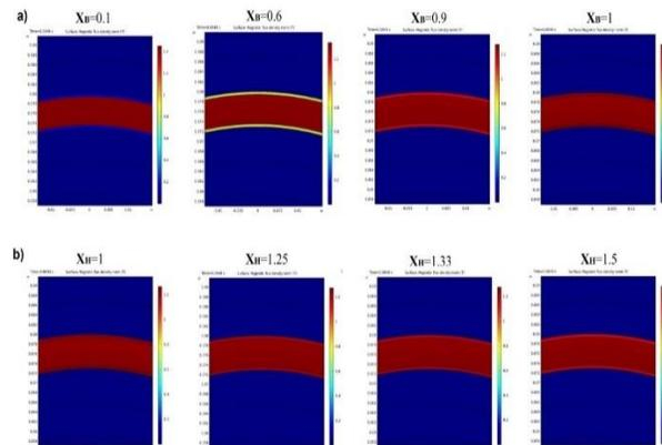
**Figure 6.** Magnetic flux density with changed coefficients: a)  $X_B = 0.1$ ,  $X_B = 0.6$ ,  $X_B = 0.9$ ,  $X_B = 1$  (no deformation) and b)  $X_H = 1$  (no deformation),  $X_H = 1.25$ ,  $X_H = 1.33$ ,  $X_H = 1.5$  when maximum value of the magnetic flux density is obtained.
