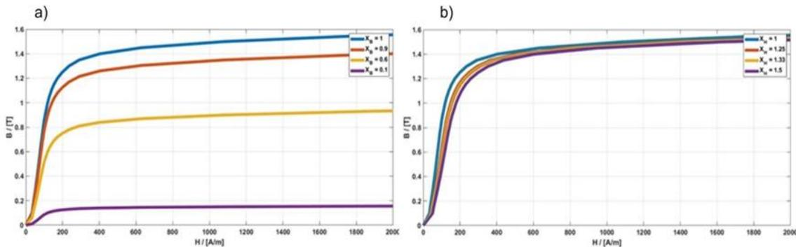
**Figure 5.** a) B-H curve with different coefficients of B when the H is fixed to healthy values b) B-H curve with different coefficients of H when the B is fixed to healthy values.
