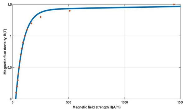
**Figure 3.** B-H curve approximation by using exponential approach for M400-50A.
