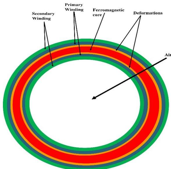
**Figure 1.** Illustration of the typical configuration of a ring-core after cutting process.
