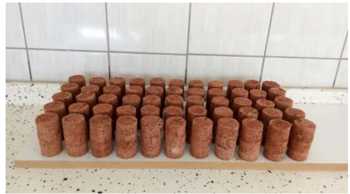
Fig. 2. The compacted cylindrical samples of the unreinforced and reinforced clayey soil
