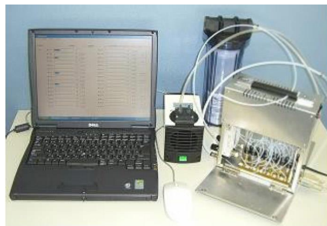
Figure 6. Photo one of the latest-version olfactory display (Nakamoto, Kinoshita, Murakami, & Yossiri, 2009).
