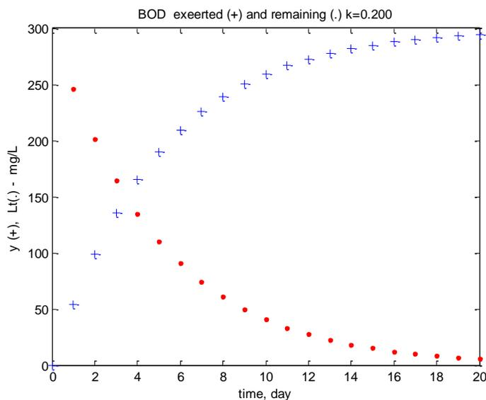
**Figure 3** Formation of the first stage BOD curve
