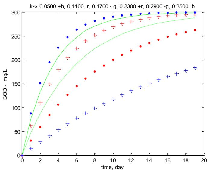
**Figure 4** Effect of the rate constant  $k$  on BOD (for a given  $L$  value)
