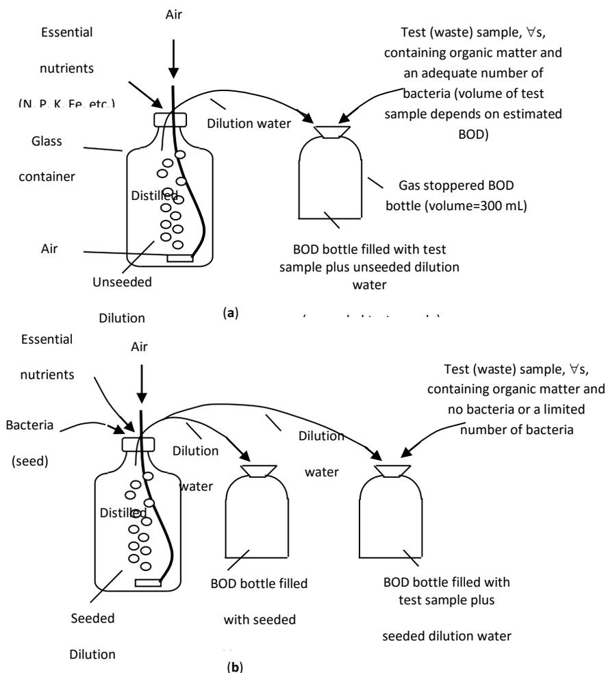
**Figure 1** Procedure for setting up BOD test bottles (a) with unseeded dilution water and (b) with seeded dilution water
