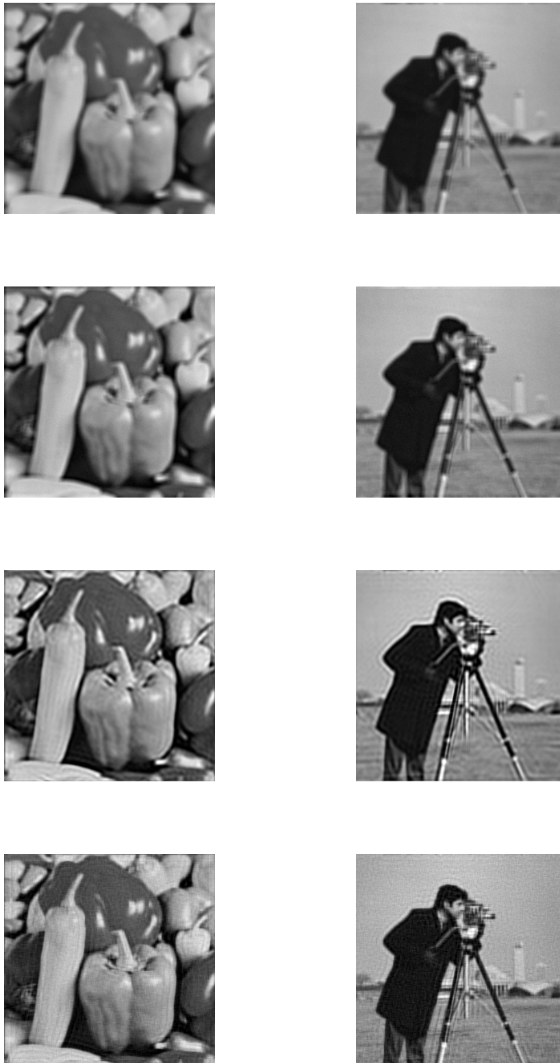
FIGURE 2. row 1: Images degraded by a Gaussian PSF with variance 5, BSNR=30, row 2: Restored images by SH-SH BD, row 3: Restored images by SH-TV BD, row 4: Restored images by Non-blind deconvolution Fast ADDM.
