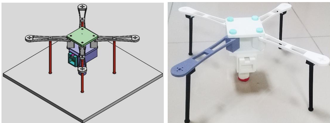
Figure 1. a) 3D model of quadcopter chasis b) 3D printed quadcopter chasis produced from PLA.
