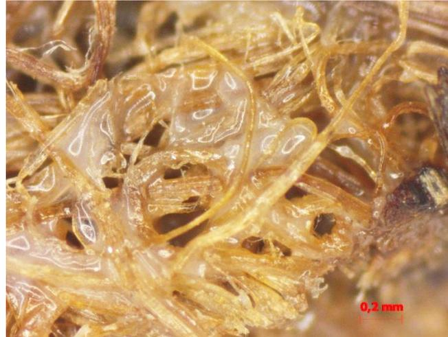
**Figure 8.** Stereomicroscope image of NF: PLA composite
