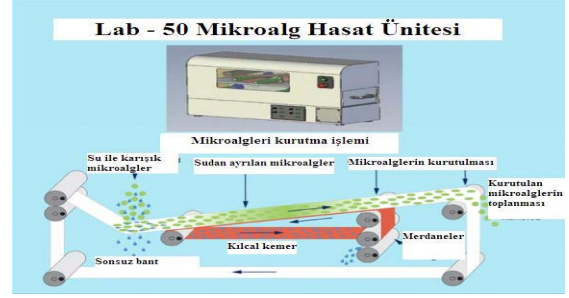
Figure 18. Lab – 50 Microalgae harvest unit process schematics (Algae Industry Magazine)
