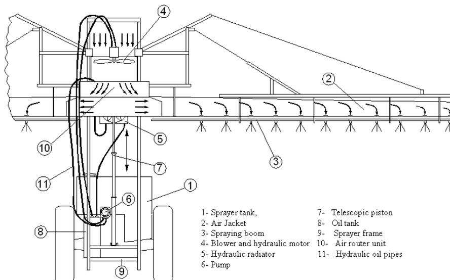
Figure 1. Schematic view of the prototype sprayer manufactured for maize plant spraying
