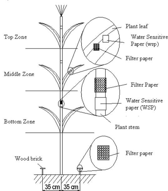
**Fig. 2. Schematic view of sampling targets on plant and ground in stage II**
