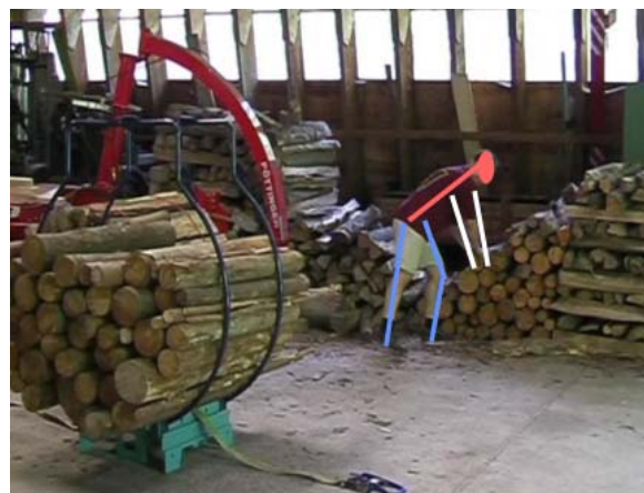
Figure 3. OWAS Code example for work postures – Code 2151
