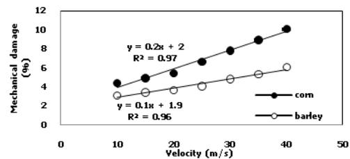
Figure 6. Effect of air velocity on mechanical damage
