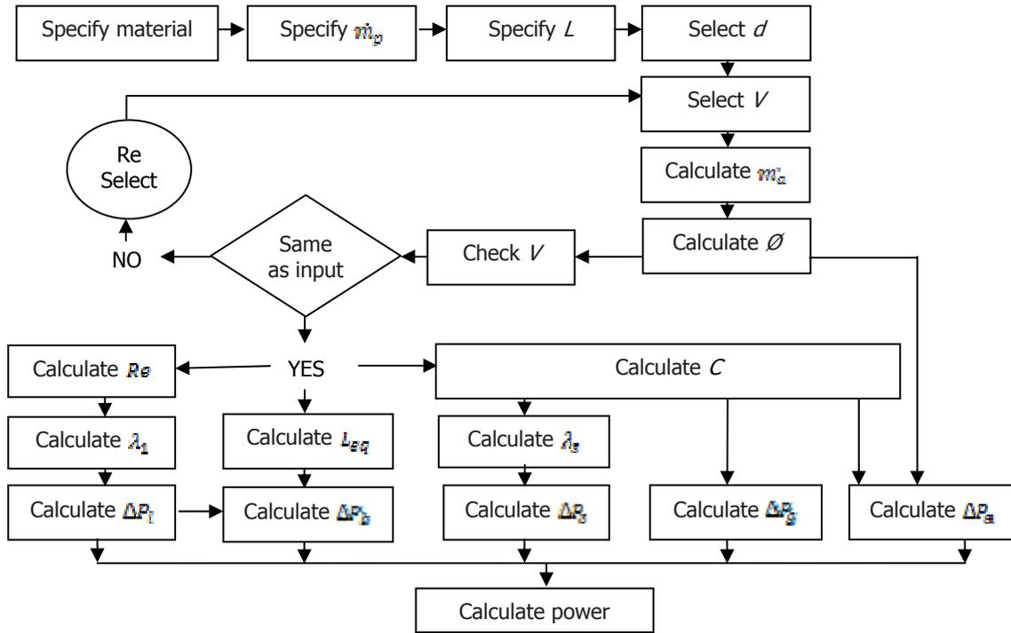
Figure 2. Logic diagram for calculating power requirement of a pneumatic conveying system
