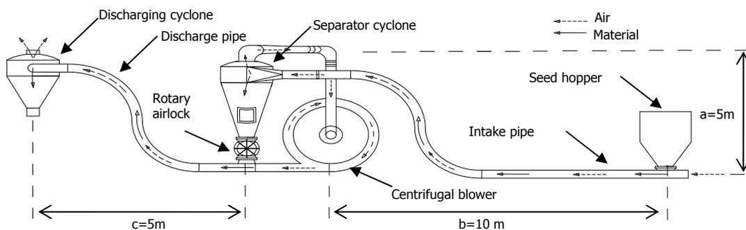
**Figure 1. Layout of the pneumatic conveying system**
