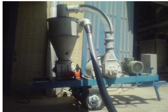
Figure 3. Pneumatic conveyer
