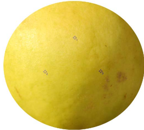
Figure 2. Selection of L*a*b* sample points by using colourmeter
