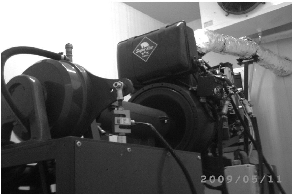
Fig.4. Cooling room and engine test mechanism
