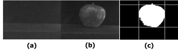
**Figure 6. Size analysis process: (a) Empty view of platform, (b) Red apple, (c) Result of size analysis**
