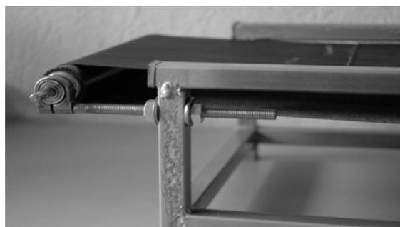
**Figure 2. Shafts of carrier band**
