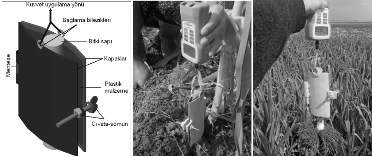
Figure 2. The apparatus which was used for measurement of pulling force of leeks and pulled plant.
