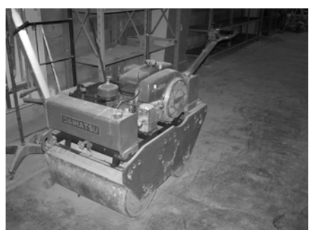
Fig. 3 Piston roller used in the preparation of the ZT-L and ZT-H plots.
