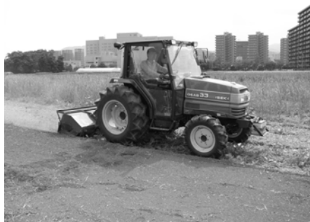
Fig. 2 Rotary tiller used in the preparation of the CT-N plots.
