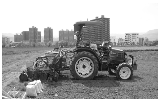
Fig. 5 Farm tractor with 4-row air seeder used in sugar beet cultivation.
