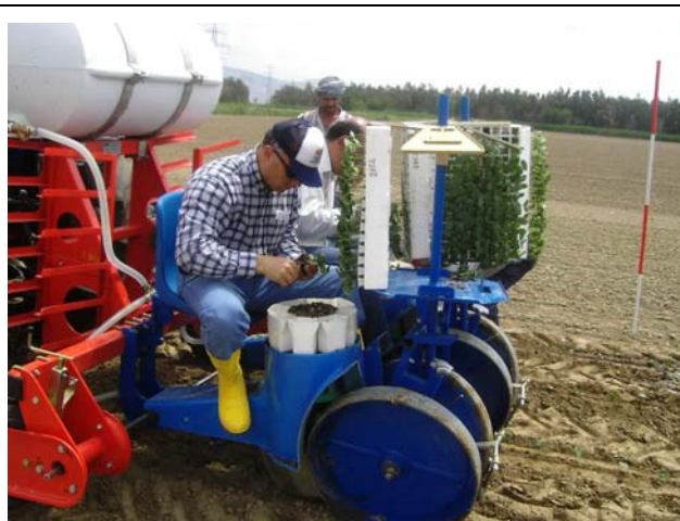
Figure 5 a. Ferrari F max model transplanting machine.
