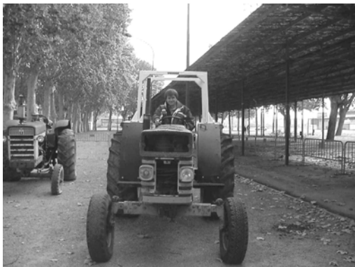
Figure 3. Improved ROPS before real overturn
