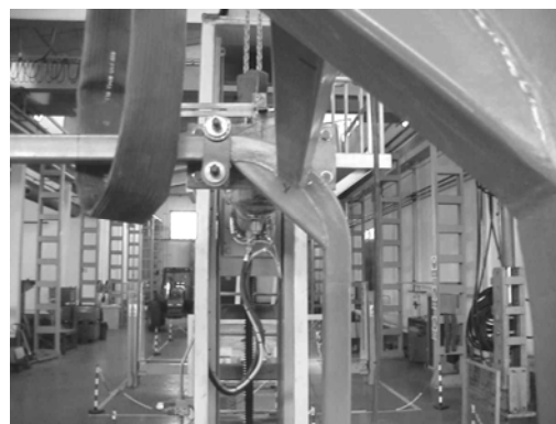
Figure 2. ROPS during rear longitudinal test
