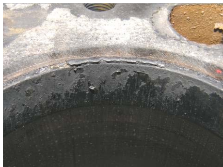
Fig. 2. Deposits on the cylinders casings
