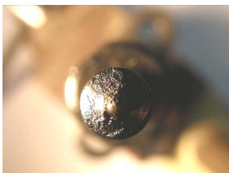
Fig. 3. Deposits in the injectors taps and on their peaks
