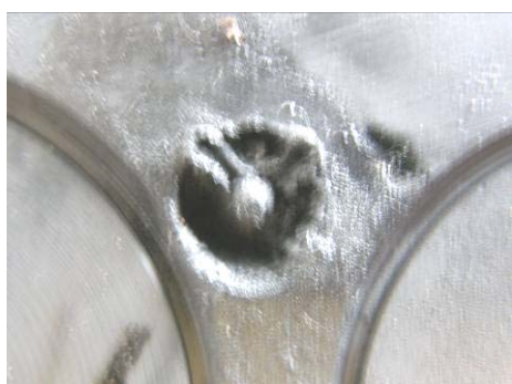
Fig. 2. Deposits on the cylinders casings
