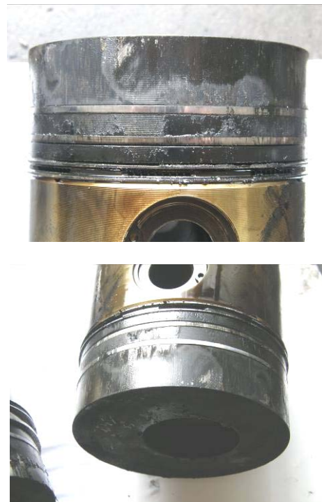
Fig. 1. Deposits which invalidate functioning of the air tightening segments
