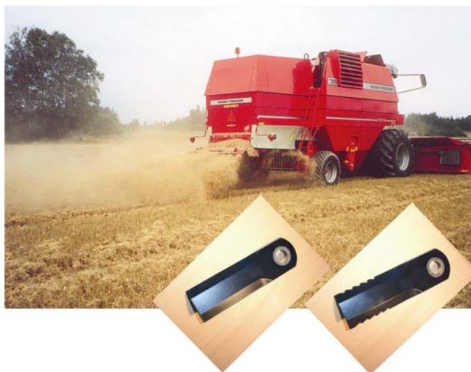
Figure 1. A total of 28 smooth reciprocating knives were mounted on the left hand side of the straw chopper and an equal number of serrated knives were mounted on the right hand side.
