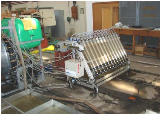
Figure 5. Equipment for determination of distribution uniformity at spraying machines in vineyards and orchards
