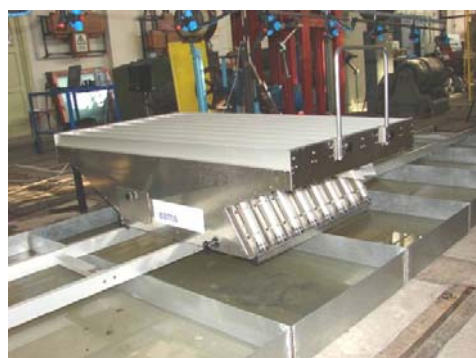
Figure 3. Equipment for verification of transversal distribution uniformity at spraying machines in base crops
