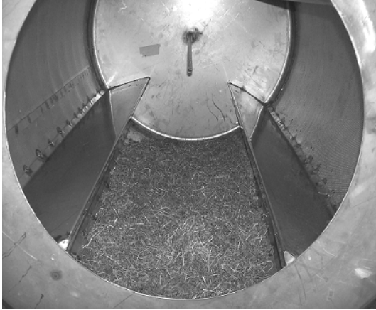
Figure 2. Inner wings of drum and pipe for temperature/RH sensor
