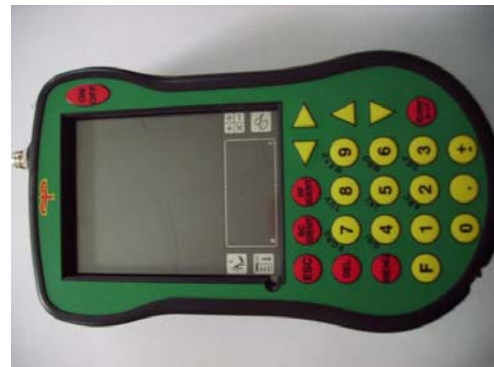
Fig. 2. Read-out device Milan MPX Mannebeck, Type 121 (photograph C. Fischer)
