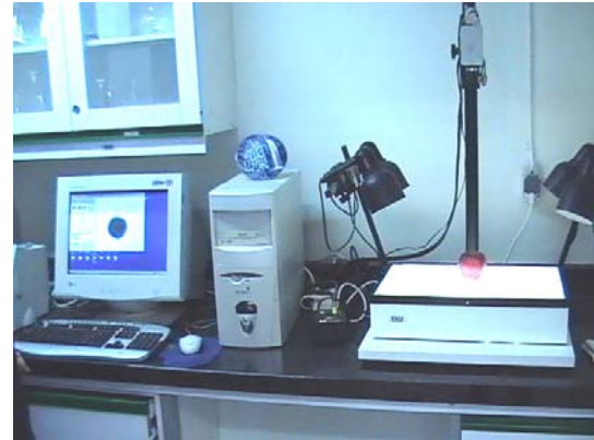
Fig. 1. Apparatus for measuring dimensional characteristics. Apple is positioned on the center of horizontal plate, directionally, under the vision of camera.
