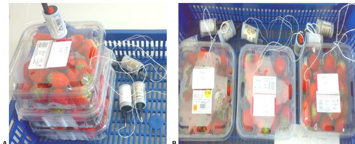
Figure 1. Cylinders of loggers were put out of punnets. Note the condensation in punnets which were in bottom (A), there is no condensation in punnet which was on top (B).
