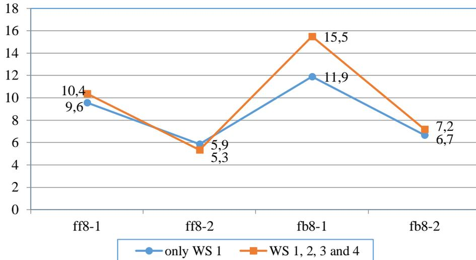
the performance of the system. Moreover, the manufacturing lead time of a system is affected not only by the number of workstations, buffer sizes, processing capacities and the number of entry workstations, but also by the layout of the system. In fact, the most important factor affecting the manufacturing lead time seems to be the layout of a system.
