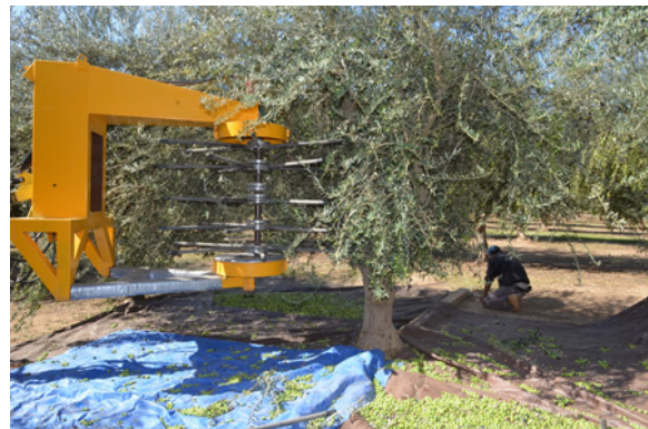
Figure 3. The "C" frame which holds the crank
