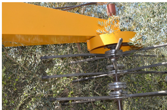
Figure 8. The shaking head presses into the tree compressing the canopy
