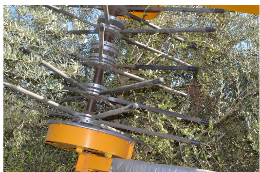
Figure 9. The interaction between the tines and larger limbs
