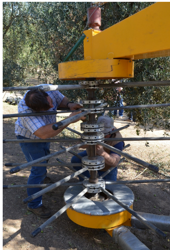
Figure 4. The crank mounted in the "C" frame
