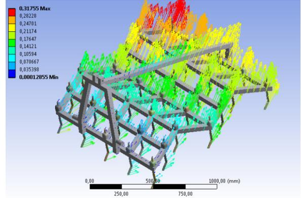
**Figure 22. Total Deformation of the Heavy Harrow Ripper Tines**
