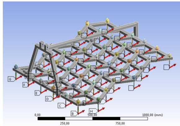
Figure 11. Loading Forces of the Light Harrow Straight Tines
