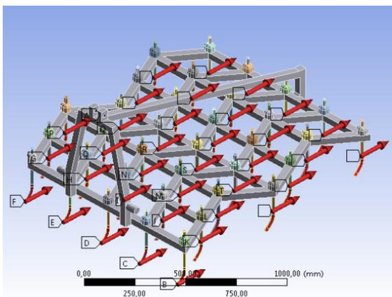
**Figure 15. Loading Forces Heavy Harrow Curved Tines**
