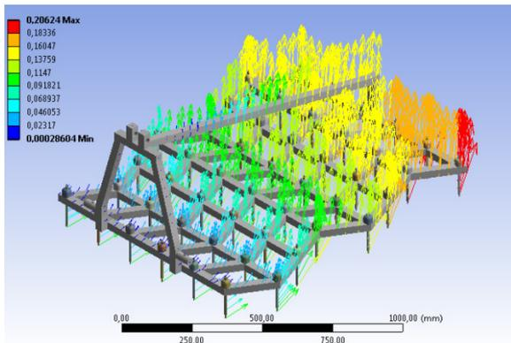
**Figure 17. Total Deformation of the Light Harrow Straight Tines**
