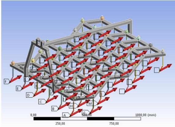
**Figure 13. Loading Forces of the Light Harrow Ripper Tines**
