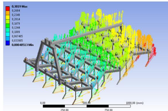
**Figure 19. Total Deformation of the Light Harrow Ripper Tines**
