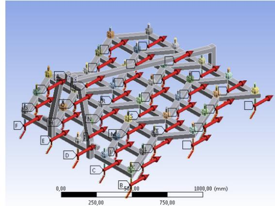
**Figure 16. Loading Forces of the Heavy Harrow Ripper Tines**
