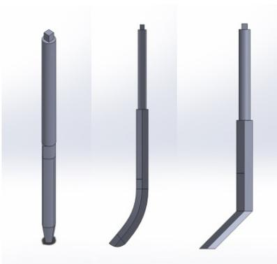
Figure 10. Tines of Heavy Harrow (Straight Tines, Curved Tines, and Ripper Teeth, Respectively.)
