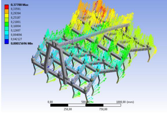
**Figure 21. Total Deformation of the Heavy Harrow Curved Tines**
