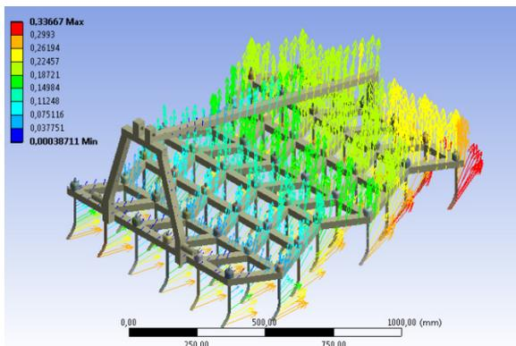
**Figure 18. Total Deformation of the Light Harrow Curved Tines**
