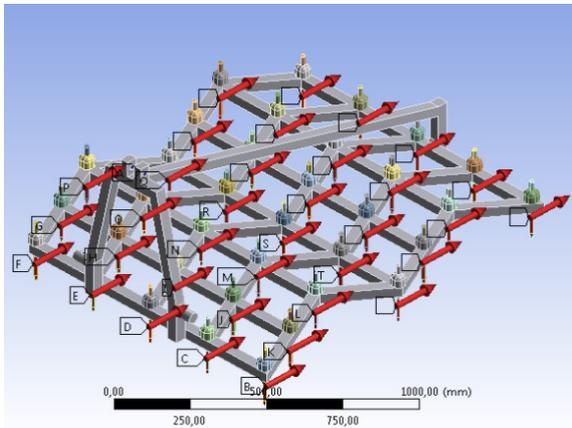
**Figure 14. Loading Forces of the Heavy Harrow Straight Tines**
