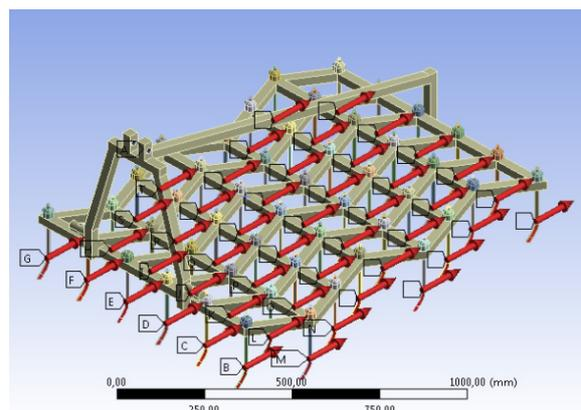
Figure 12. Loading Forces of the Light Harrow Curved Tines
