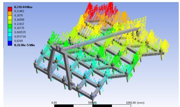
**Figure 20. Total Deformation of the Heavy Harrow Straight Tines**
