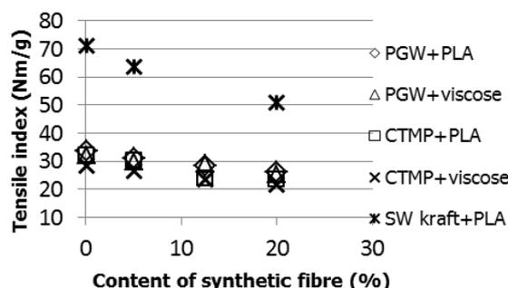
**Figure 2. Tensile index of the sheets as a function of the synthetic fibre content. With PGW and CTMP the standard deviation ranged from 0.8 to 2.2 Nm g<sup>-1</sup> and in SW kraft from 2.0 to 2.8 Nm g<sup>-1</sup> (Asikainen & Korpela 2014)**
