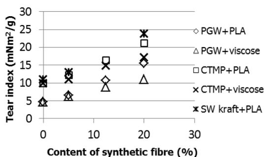
**Figure 1. Tear index of the sheets made with a minor share of synthetic fibre. With PLA the tear index increased 117% in CTMP and 243% in PGW stock, while with the viscose fibre the index increased 77% and 141% respectively. In softwood kraft the tear index increased 118% (Asikainen & Korpela 2014)**
